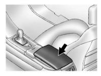
The center console has an upper and lower storage area. To access, lift the levers on either side of the center console. There is an additional storage area behind the center console. To access, push the cover.
